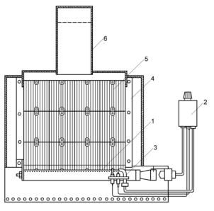
• Thermoelectric generator is built into heating boiler and comprises several basic parts: heat source, thermopiles, heat and smoke fumes input and output systems.
