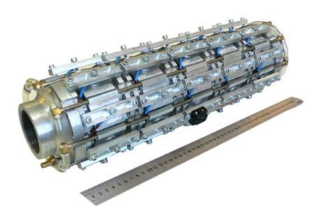
• Thermoelectric generator is composed of thermoelectric generator modules, hot gas heat sinks with variable heat exchange coefficients, liquid heat exchangers for heat disposal and hydro and electric connections.
