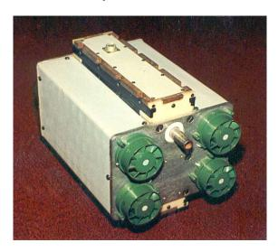
• The conditioner is made as thermoelectric thermal pump of the water «water-air» type. The device includes water heat exchangers, thermoelectric modules, radiometers of the sink system as well as a pump and a fan for fluid circulation.
