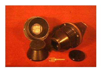
100 mV/J is the best energetic sensitivity multielement laser radiation detectors.
